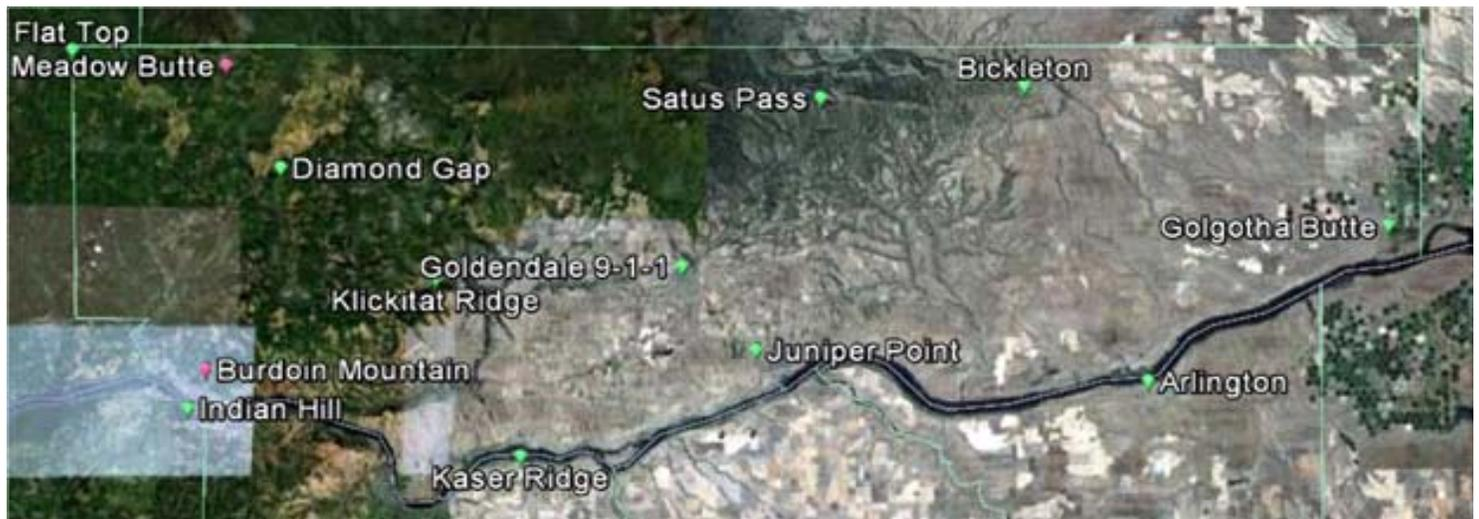
The county is long and narrow with approximately 1,900 square miles of area. The deep Columbia River Gorge made providing radio coverage along the state highway and the towns along the river difficult. In the end, the system designed and implemented has 11 sites and eight channels with simulcast used throughout the network as shown in the map above.
